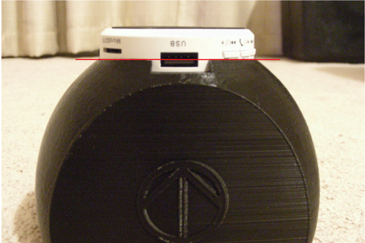
Speaker placed in test model. The red line is where you should align the USB port to the slot, using the rectangular protrusion inside the slot.
